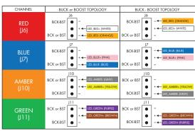
Refer to this image to connect the LED Daughter Card Interface on the main board and the Main Board Interface on the daughter board. Note that the Buck or Boost Topology is required for the onboard firmware to work properly
