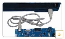
Connect the main board to the PC using the USB cable provided with the kit
