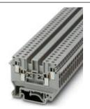
Single-level terminal block with two-sided double connection, test socket screws, cross section:  $0.2 - 2.5 \text{ mm}^2$ , AWG: 30 - 10, width: 6.2 mm, color: gray
