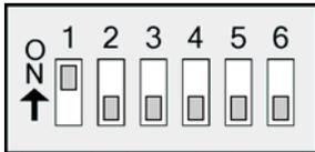
DIP Switch settings are read and applied only while powering-on.
