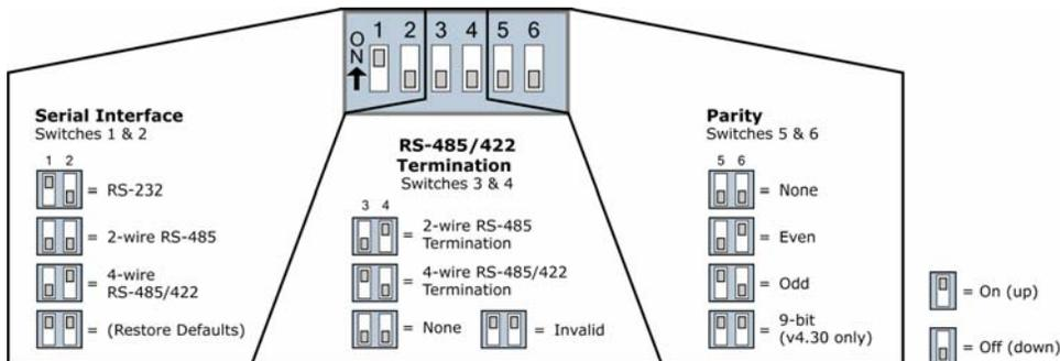
Refer to table in the Automatic DIP Switch Configurations section [next page] for more information regarding configurations triggered by the DIP Switch.
