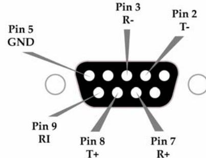
Termination is the 120 Ω resistor between T+ and T-.
