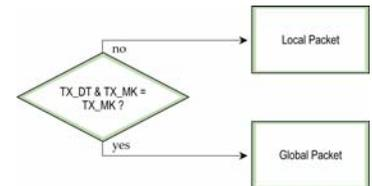
A receiving module will only accept a packet if a packet is addressed to it (either as a global or local packet). The RX module makes this determination by inspecting the destination address of the RF packet and comparing it to its own address and mask. The Destination Address of the TX module is logically "ANDed" with the Address Mask of the RX module.
