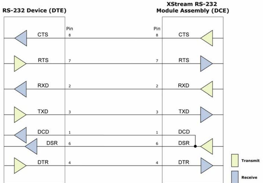
**Wiring Diagram: DCE Module Assembly to an RS-232 DCE Device**
