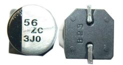
Rated for 125°C, type HZC combines the advantages of aluminum electrolytic and aluminum polymer technology. These hybrid capacitors have the ultra-low ESR characteristics of conductive aluminum polymer capacitors packaged in a V-chip, SMT case with high capacitance and voltage ratings that were previously available only in aluminum electrolytic technology. Applications for type 125°C hybrid capacitors include a variety of industrial power conversion, lighting control and automotive applications.
